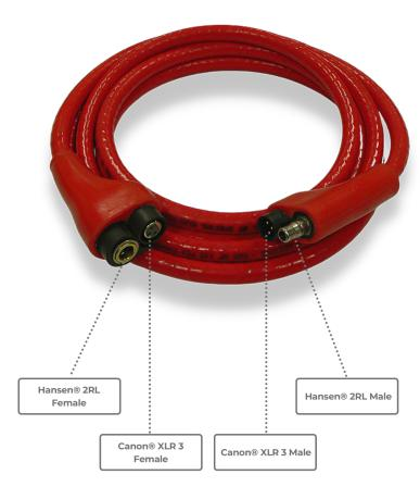
**APPLICATIONS:** · Nuclear, Industrial · Radiation Personal Protection Equipment PPE · Vault Suit Breathing Air Hose **Chemical Plants CONNECTOR STYLE:** Standard: Hansen® 2RL, and Canon® XLR 3 By Special Order Optional: **RATINGS:** Working Pressure: 125lbs @ 68°F Air Flow @ 75psig: 28scfm (13.2L/sec) **CHEMICAL RESISTANCE:** Strong Acids Excellent Weak Acids Good Strong Alkalis Excellent Weak Alkalis Good Aliphatics Good
